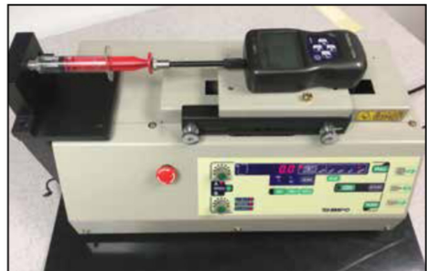
Shimpo Equipment Testing Compression Force on Syringe's Needle
