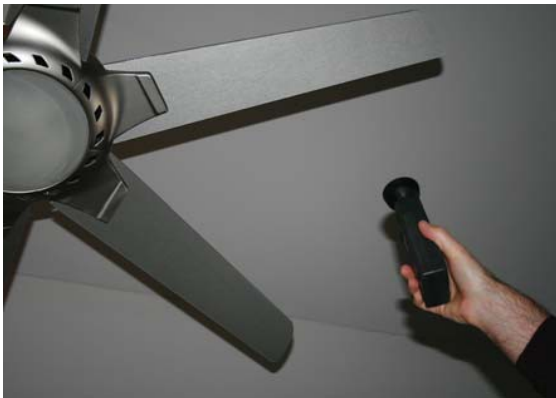
ST-1000 Checking Fan Speed and Balance
