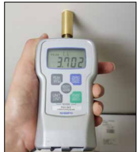
Performing Puncture Test on Drywall
