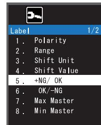
7 Setting work lower tolerance limit value.
