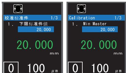
12 Set 「Min Master」 on measurement jig. After the indicators stabilizes, press **ENT**.
