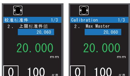
13 Set 「Max Master」 on measurement jig. After the indicators stabilizes, press **ENT**.
