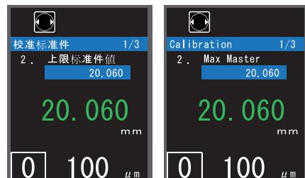
14 Check the display of 「TFT LCD」. 「MAS OK」 Mastering is successful. Proceed to measurement.
